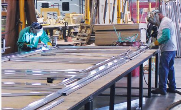
Spyder features aluminum framing laminated with block foam insulation, true gel coat fiberglass exterior, and designer interior décor panels.
